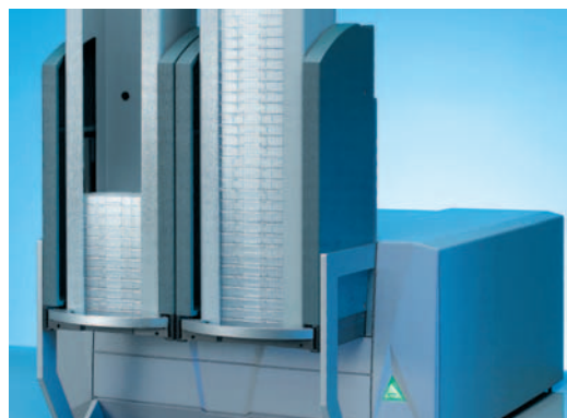
Integrated stackers with compact design for minimum increase in footprint.
